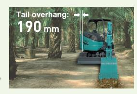
The tail overhang is 196 mm, which is within 10 % of the machine width complying with the Japanese definition of SR (Short Radius).
