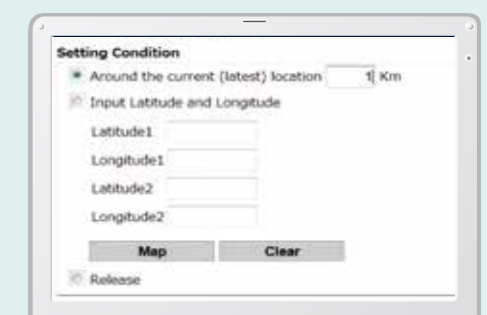
Alarm for outside of reset area
