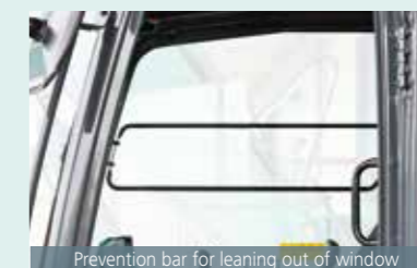
Prevention bar for leaning out of window
