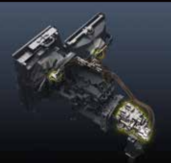
Hydraulic drive optimizes the cooling fan rotation speed to improve fuel economy and reduce noise. Also, the independent oil cooler fan better matches cooling to the hydraulic oil temperature, for optimal oil temperature control.
